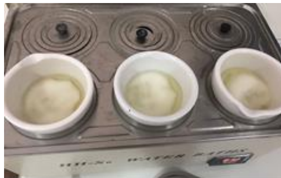
Figure 1. Fatty Phase melting in water bath at 70-75°C.
